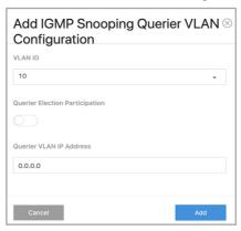
Querier Election Participation does not need to be enabled if you are manually setting the Core switch in the network as the querier, and you're leaving querier disabled on the edge switches. Leave Querier VLAN IP Address at 0.0.0.0
